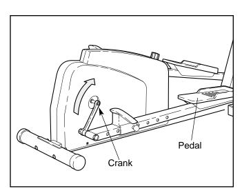
To dismount the REBEL, allow the pedals to slowly come to a stop. Important: The REBEL does not have a free wheel; the pedals will continue to move until the flywheel stops. When the pedals are stationary, step off the highest pedal first. Then, step off the lowest pedal.
